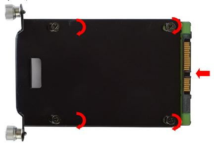
Insert the mounting bracket of the hard disk into the case and lock the fixed screws on both sides.
