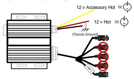
The yellow ignition wire is used to detect the ignition signal. We strongly suggest you connect it with the "RUN" terminal of the ignition switch.
