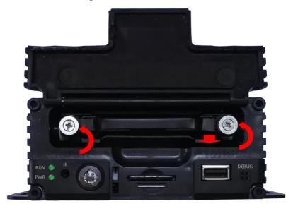
Insert the hard drive into the bracket as shown below and secure the 4 fixed screws. (These screws were shipped with the DVR and are in the accessory box.)
